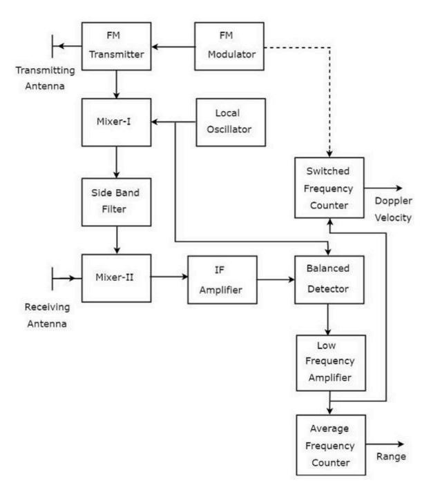
**FMCW Radar** contains two Antennas — transmitting Antenna and receiving Antenna as shown in the figure. The transmitting Antenna transmits the signal and the receiving Antenna receives the echo signal.
