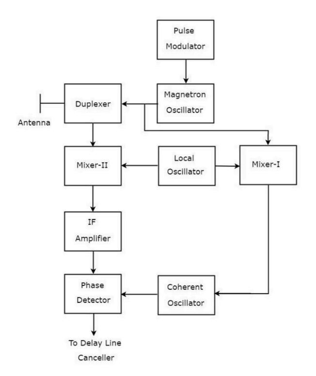
As shown in the figure, MTI Radar uses the single Antenna for both transmission and reception of signals with the help of Duplexer. The **operation** of MTI Radar with power oscillator transmitter is mentioned below.
