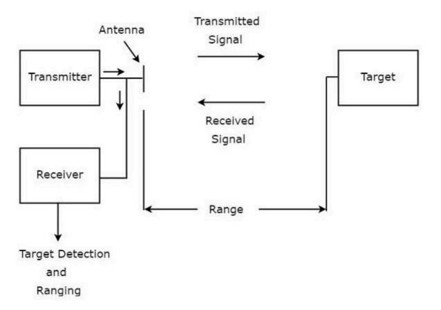
As shown in the figure, Radar mainly consists of a transmitter and a receiver. It uses the same Antenna for both transmitting and receiving the signals. The function of the **transmitter** is to transmit the Radar signal in the direction of the target present.
