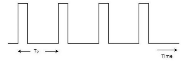
As shown in the figure, Radar transmits a periodic signal. It is having a series of narrow rectangular shaped pulses. The time interval between the successive clock pulses is called **pulse repetition time**,  $T_P$ .
