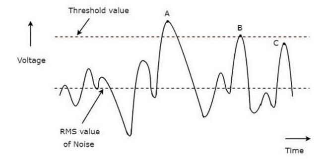
A **typical waveform** of the Radar receiver is shown in the above figure. The x-axis and y-axis represent time and voltage respectively. The rms value of noise and threshold value are indicated with dotted lines in the above figure.
