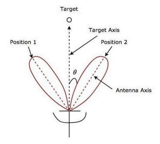
As shown in the figure, Antenna beams switch between Position 1 and Position 2 alternately. Angular error  $\theta$  is indicated in the above figure. Sequential lobing gives the position of the target with high accuracy. This is the main **advantage** of sequential lobing.
