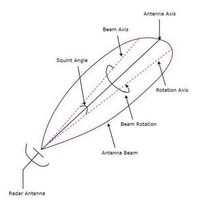
**Squint angle** is the angle between beam axis and rotation axis and it is shown in the above figure. The echo signal obtained from the target gets modulated at a frequency equal to the frequency at which the Antenna beam rotates.
